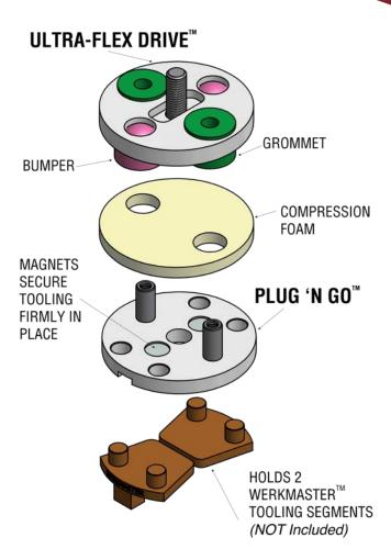
Just PLUG 'N GO. When it comes to all WerkMaster machines, putting on and removing your tooling is a breeze.
