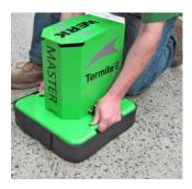
Remove the handle and you have a high performance hand grinder for polishing surfaces like countertops or for getting into hard to reach areas
