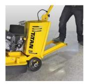
EZ Bak tilt feature allows for operators weighing 135 pounds or more to easily tilt back the machine to change tooling and for transport
